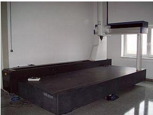
MITUTOYO 3D CNC Messmaschine **Crysta Apex C 123010**
